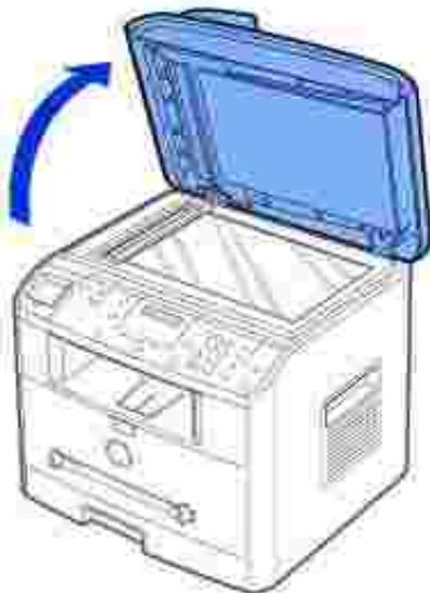
3. Wipe the surface of the scanner glass and ADF glass until it is clean and dry.
